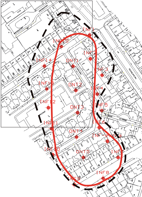
Figure 2. Layout of the 16 infiltration (INF) and 5 extraction (ONT) wells, including the plume delineation.
